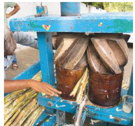
Though clearly hand carved, those helical gears seemed to mesh quite smoothly
